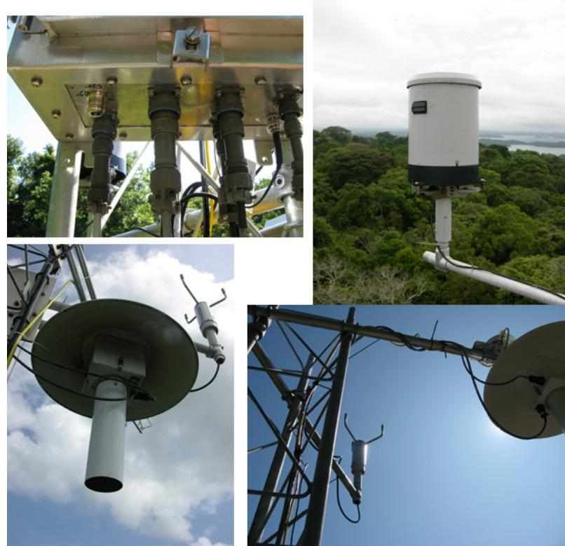
The SIGEO-CTFS stations comprise several sensors recorded automatically by a CR1000 datalogger (Campbell Scientific) at 5 min time interval. These sensors include:
